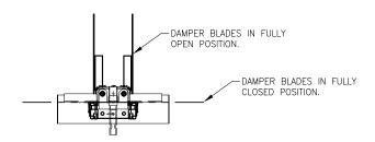
2. ONCE THE BLADE IS IN OPEN POSITION, MOUNT DIRECTLY ONTO PLENUM BY CLIPPING TO INLET NECK. BLADES OPEN TO THE UPSTREAM DIRECTION.
